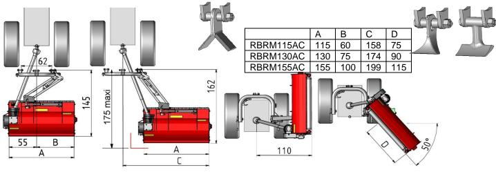
Serial Assembly with Y-knives, option assembly with paddles or hammers
